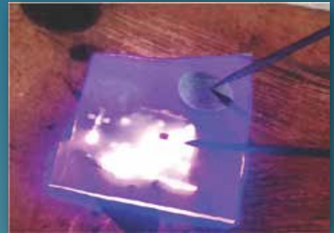
GaN LED with graphene top electrode
